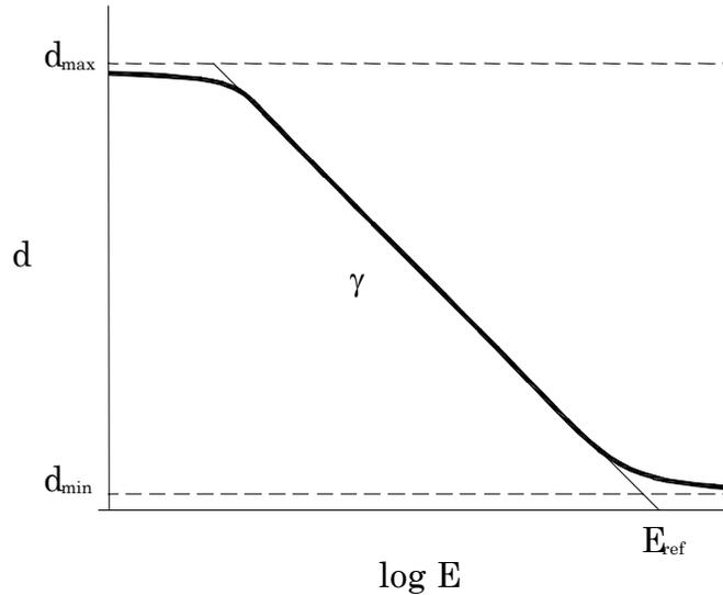
Here  $d$  is the photographic density, with  $d = 0$  meaning transparent film (or fully white) and as  $d$  becomes larger, transparency decreases (the film becomes darker).  $E$  is the light exposure the film receives, measured in candela-sec/m<sup>2</sup> or similar units.  $(-\gamma)$  is the slope of the straight-line portion of the S-curve.  $E_{\text{ref}}$  is the exposure for which  $d = 0$  when the straight-line portion is extrapolated through the  $\log E$  axis.
